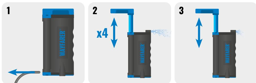
1. Remove the Out Hose and use your Wayfarer™ as normal. During the pumping cycle remove the Scavenger In Hose from the spigot.
